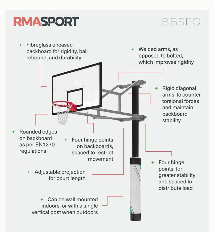
A high quality side folding system for use indoors or out, designed for performance, strength and durability.
